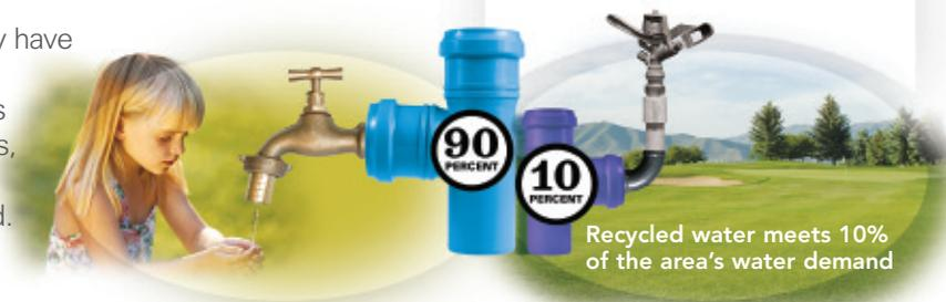
Purple pipe is used to isolate recycled water.
